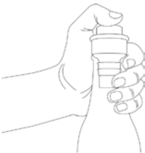
Press the stopper repeatedly to extract the air
